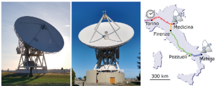
Figure: The telescopes at Medicina and Matera, and the overview map with the fiber link (image credits: photos: J. Roda, INAF/IRA (Medicina), M. Sicillani De Cumis, ASI (Matera); map: figure adapted from 1 )
