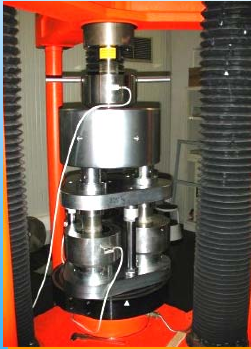
Fig.7: Calibration of the INRIM - 3 MN Build-up system on the INRIM - 1 MN DWM
